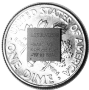
Figure 8: Size comparison of an MEMS acceleration sensor
