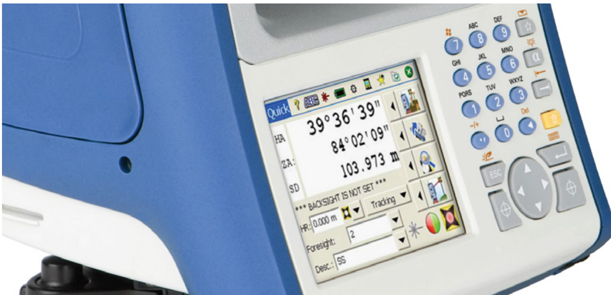
Figure 15: FOCUS 30 control unit with Survey Pro application software
